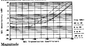
Note: System performance in 2.92mm (K) connectors is provided to indicate typical uncertainty using 2.92mm adapters after 2.4mm calibration. Performance is not verifiable due to lack of traceable standards in K-connectors. These curves indicate worst-case sums of errors; typical uncertainties are less than half the values indicated.
