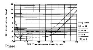
1 Reference power level is -5 dBm into the test port.
